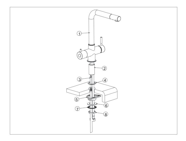
15. Drill the chosen position with a 32mm drill bit (or use pre-drilled sink hole). It is recommended to dot punch a sink top before actually drilling to prevent your drill from slipping.
