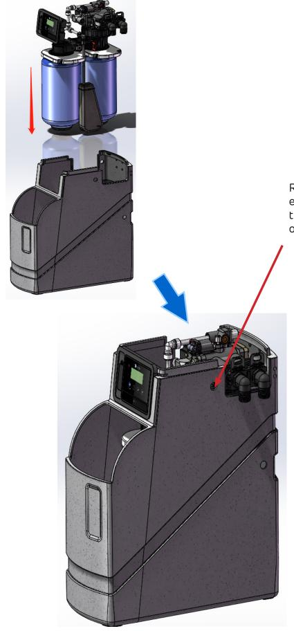
Remove the drain elbow from the side of the cabinet and place it on the opposite side.
