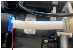
Using the supplied fittings and tubing (8cm), attach the air check to the valve, using the push-fit connector and placing the blue clip back on (as pictured).
