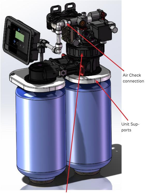
Undo the large nut at the base of the main valve body, take out the valve and twist 180 degrees until the connections are on the other side.
