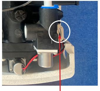
Remove the small grey clip from the air check connector.
