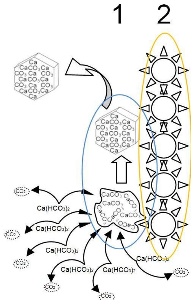
**FILTERSORB® SP3** formed crystals can sustain a temperature up to 380°C, before a structural breakdown back to the calcite form. This property of the transformed hardness makes the treated water perfect for hot water applications and boilers.
