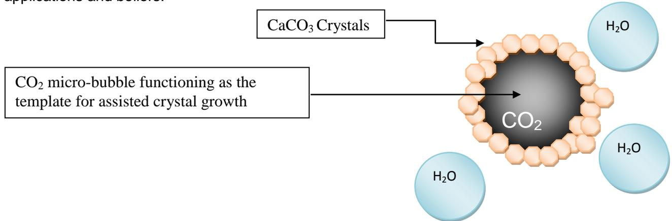
During the flow some of the micro-bubbles are losing a small amount of CO<sub>2</sub>, which diffuses rapidly in water and interact with surface scale, especially in closed spaces (pipes, boilers, etc). As a result, the scale which is already present on these surfaces is slowly softened and removed.
