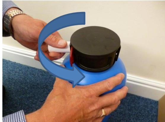
7. Remove head complete with internal tube. Be aware of slight water spillage here.
