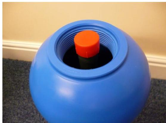
9. Clean top of vessel where head 'o' ring joins for seal and apply a small amount of Vaseline to 'o' ring and head seal area to help the heads main 'o' ring to seal.
